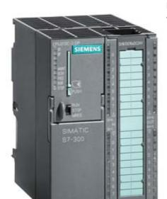
SIMATIC S7-300, CPU 313C-2 DP Compact CPU with MPI, 16 DI/16 DO, 3 high-speed counters (30 kHz), integrated DP interface, Integr. power supply 24 V DC, work memory 128 KB, Front connector (1x 40-pole) and Micro Memory Card required
