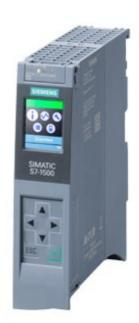
SIMATIC S7-1500, CPU 1511-1 PN, Central processing unit with working memory 150 KB for program and 1 MB for data, 1. interface: PROFINET IRT with 2 port switch, 60 NS bit-performance, SIMATIC memory card necessary
