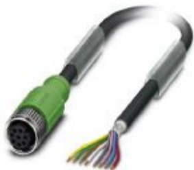
Sensor/actuator cable, 8-position, PUR halogen-free, black-gray RAL 7021, shielded, free cable end, on Socket straight M12, coding: A, cable length: 10 m
