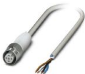
Sensor/actuator cable, 4-position, PP-EPDM halogen-free, gray RAL 7035, free cable end, on Socket straight M12, coding: A, cable length: 5 m, Hygienic design, with high-grade steel knurl
