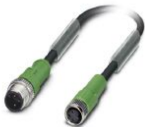
Sensor/actuator cable, 3-position, PUR halogen-free, black-gray RAL 7021, Plug straight M12, coding: A, on Socket straight M8, cable length: 1.5 m
