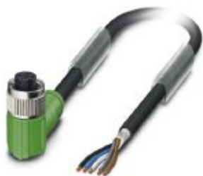
Sensor/actuator cable, 5-position, PUR halogen-free, black-gray RAL 7021, shielded, free cable end, on Socket angled M12, coding: A, cable length: 1.5 m
