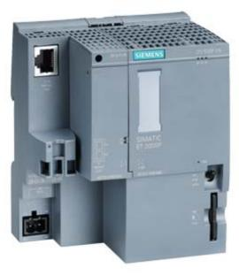
SIMATIC DP, CPU 1512SP-1 PN for ET 200SP, Central processing unit with Work memory 200 KB for program and 1 MB for data, 1st interface: PROFINET IRT with 3-port switch, 48 ns bit performance, SIMATIC Memory Card required, BusAdapter required for Port 1 and 2
