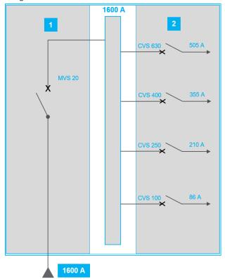
The product used for the analysis is the typical PrismaSet M Aluminium Busbar Floor standing switchboards 1600A product, which is comprised of the following commercial references:
