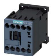
power contactor, AC-3e/AC-3, 16 A, 7.5 kW / 400 V, 3-pole, 24 V DC, with integrated diode, auxiliary contacts: 1 NC, screw terminal, size: S00  $\,$
