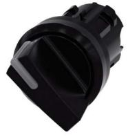
Illuminable selector switch, 22 mm, round, plastic, black, Selector switch short, 2 switch positions O<I, momentary contact type, Actuating angle  $45^\circ$ , 10:30h/12h
