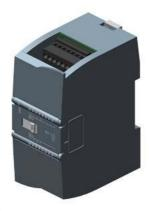
SIPLUS S7-1200 SM 1222 8DQ based on 6ES7222-1BF32-0XB0 with conformal coating, -40...+70 °C, start up -25 °C, digital output 8 DQ, 24 V DC, transistor 0.5 A
