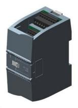
SIPLUS S7-1200 SM 1234 4Al/2AQ based on 6ES7234-4HE32-0XB0 with conformal coating, -40...+70  $^{\circ}$ C, start up -25  $^{\circ}$ C, analog I/O +/-10 V: 14-bit resolution 0-20 mA: 13-bit resolution
