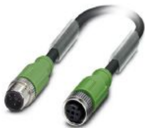
Sensor/actuator cable, 4-position, PUR halogen-free, black-gray RAL 7021, shielded, Plug straight M12, coding: A, on Socket straight M12, coding: A, cable length: 0.3 m
