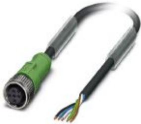
Sensor/actuator cable, 5-position, PUR halogen-free, black-gray RAL 7021, free cable end, on Socket straight M12, coding: A, cable length: 5 m
