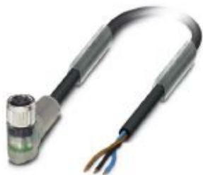
Sensor/actuator cable, 3-position, PUR halogen-free, black-gray RAL 7021, free cable end, on Socket angled M8, with 2 LEDs, cable length: 5 m
