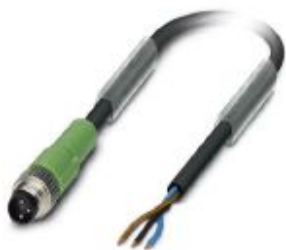
Sensor/actuator cable, 3-position, PUR halogen-free, black-gray RAL 7021, Plug straight M8, on free cable end, cable length: 3 m
