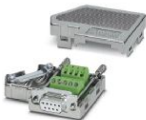
D-SUB connector, 9-pos. female connector, two cable entries < 35°, universal type for all systems, pin assignment: 1, 2, 3, 4, 5, 6, 7, 8, 9 to one screw connection terminal block
