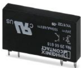
Plug-in miniature solid-state relay, input solid-state relay, 1 N/O contact, input: 24 V DC, output: 3 - 48 V DC/100 mA
