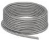
PROFINET power cable, 5x 2.5 mm<sup>2</sup>, stranded (7-wire), outer sheath: PVC, outside diameter 11.8 mm, RAL 7001 (silver gray), oil-resistant, by the meter
