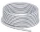
PROFINET power cable, 5x 2.5 mm<sup>2</sup>, stranded (7-wire), outer sheath: PVC, outside diameter 11.8 mm, RAL 7001 (silver gray), oil-resistant, cable ring: 100 m
