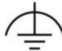
Connection of the protective equipotential bonding conductor
