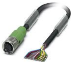
Sensor/actuator cable, 17-position, PUR halogen-free, black RAL 9005, free cable end, on Socket straight M12 SPEEDCON, coding: A, cable length: 1.5 m
