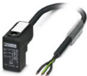
Sensor/actuator cable, 3-position, PUR halogen-free, black-gray RAL 7021, free cable end, on Valve connector C (8 mm), with 1 LED, connected with Z diode, cable length: 3 m
