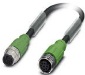
Sensor/actuator cable, 8-position, PUR halogen-free, black-gray RAL 7021, shielded, Plug straight M12, coding: A, on Socket straight M12, coding: A, cable length: 3 m
